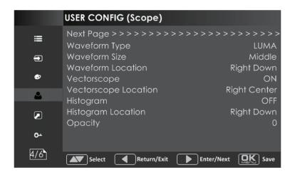
Set the location of waveform, vector scope and histogram by USER CONFIG → Waveform Location/ Vector scope Location/ Histogram Location separately, the available locations on the screen are as shown in following figure:
