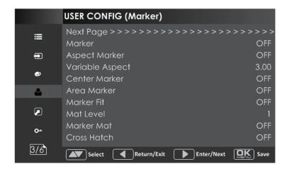
**Marker:** Set whether to show all of the markers. It is the main switch for area marker, center marker and safety marker.
