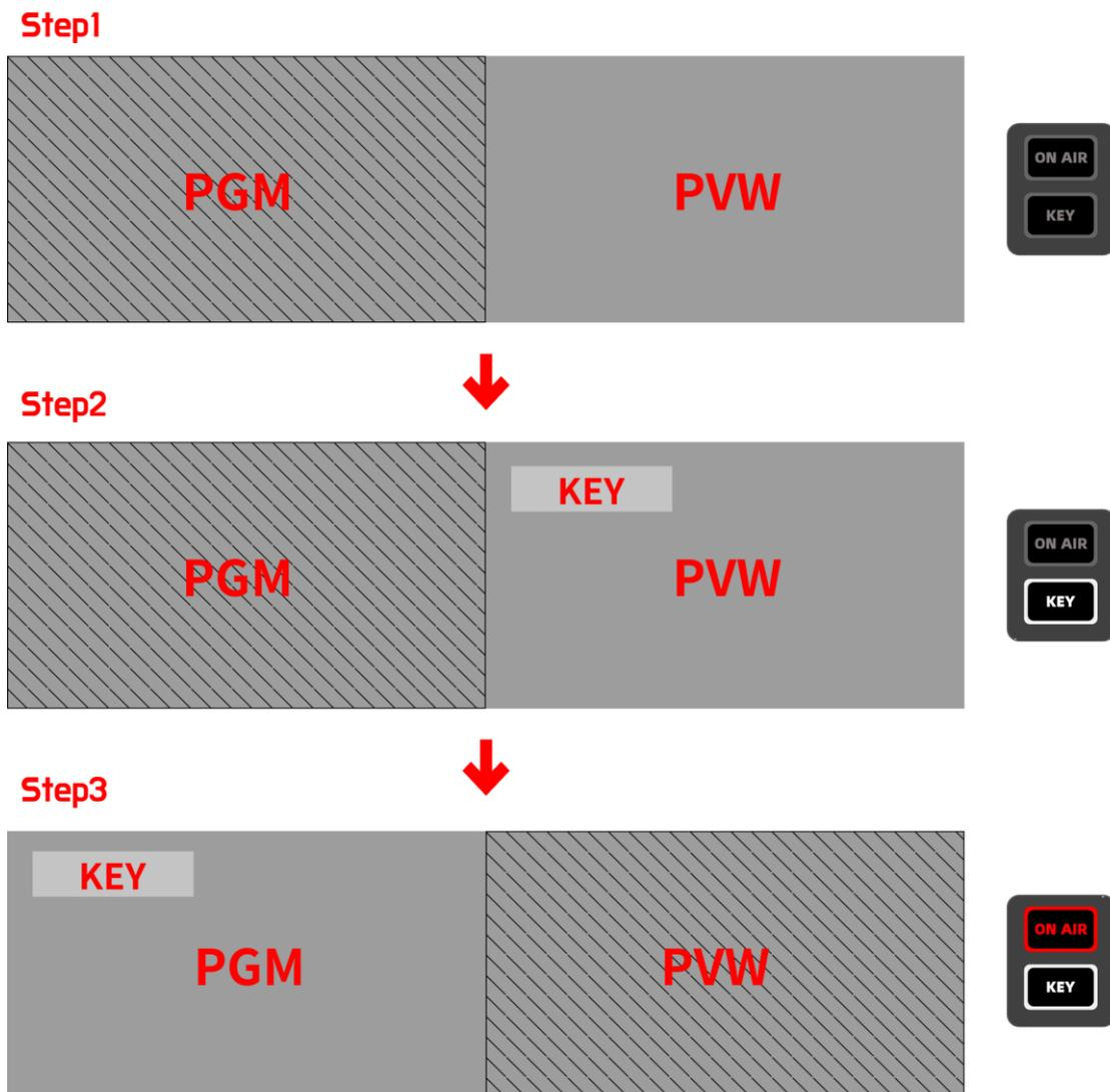
**Figure 4.1-53 Before and After Upstream Key Transition-Example2**
