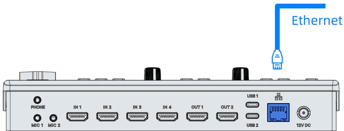
**Figure 4.1-73 Ethernet Connection**
