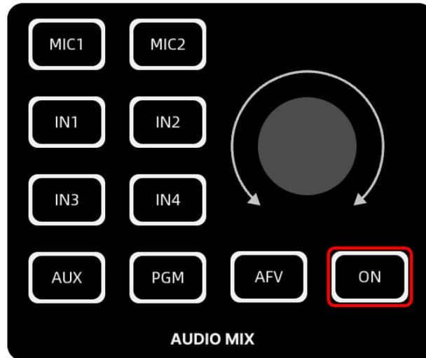
**Figure 4.1-60 On Button in Audio Mix Area**
