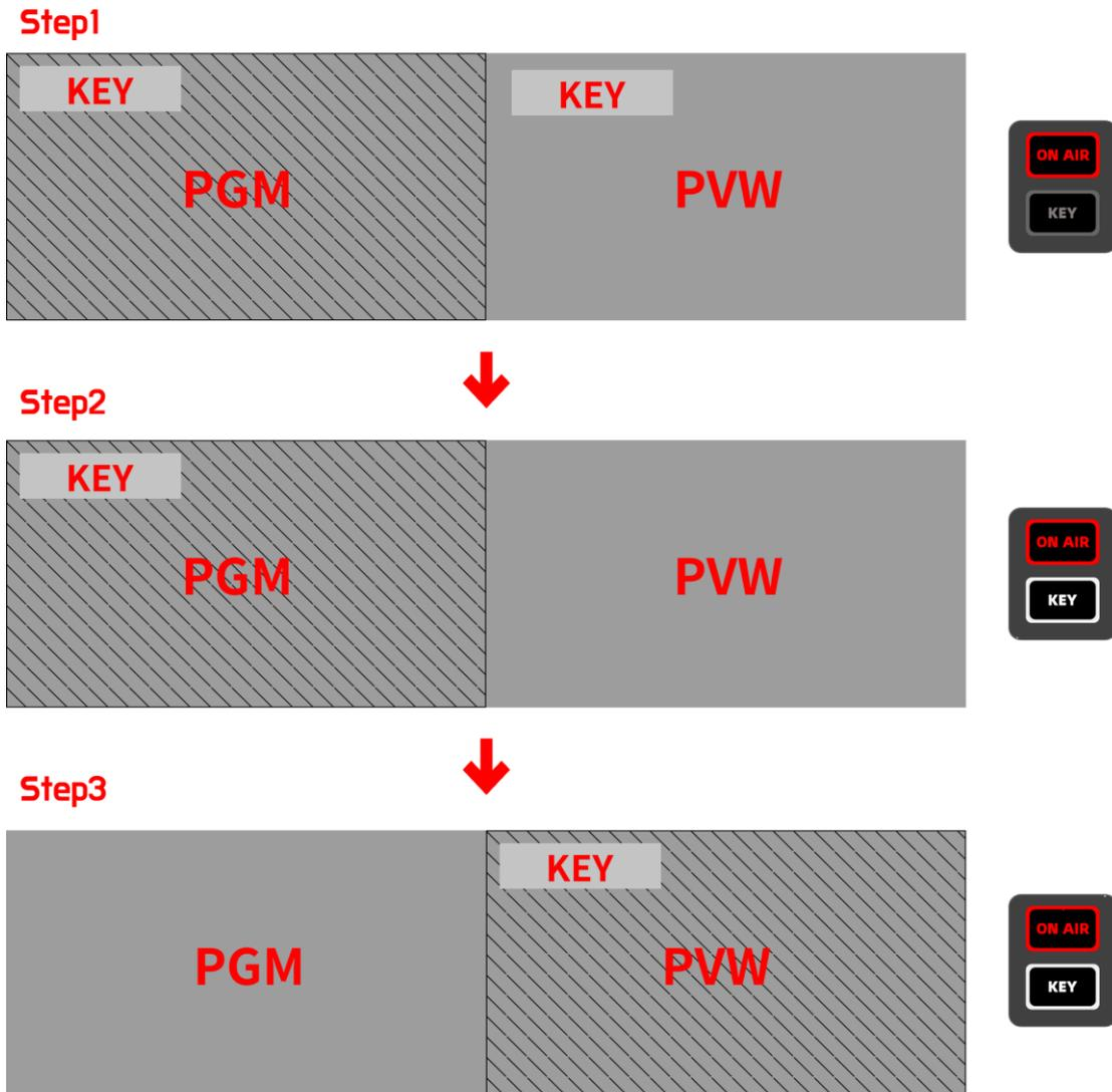
Figure 4.1-52 Before and After Upstream Key Transition-Example1
