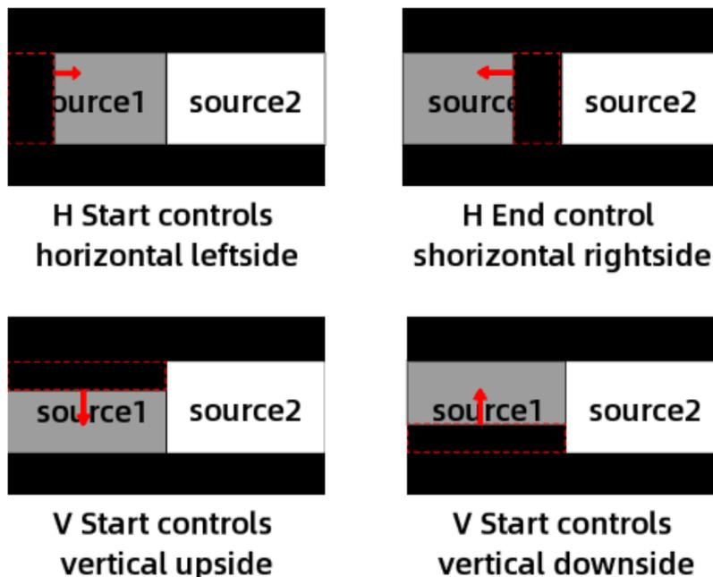
**Figure 4.1-27 Crop Splicing Display Example**
