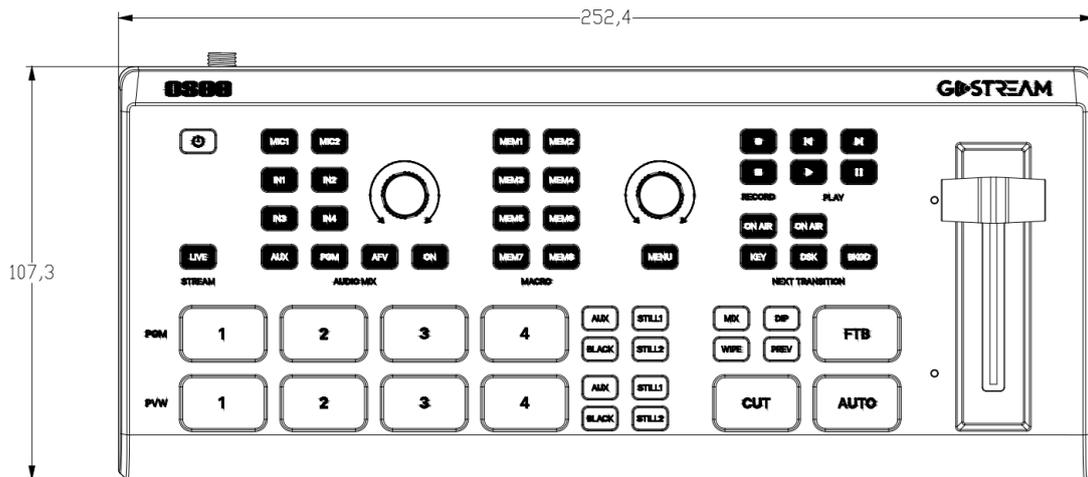
**Figure 6-1 Front Panel(Unit: mm)**
