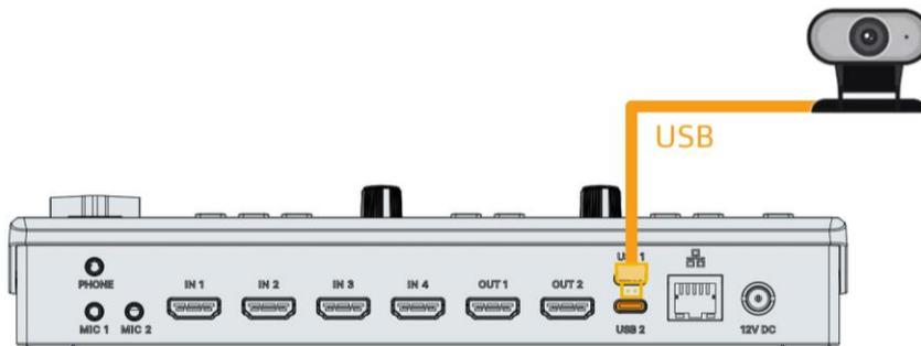
**Figure 4.2-6 Connect a Webcam as AUX Source**
