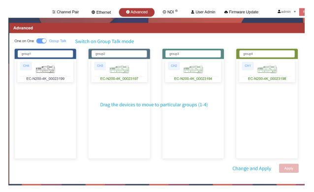
When several camera adaptors are in a same group, press any of the camera numbers on the intercom control panel, the other cameras in the same group will be actived automatically, and all the cameras in this group can talk with director simultaneously.
