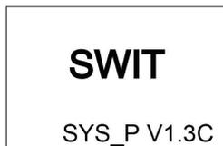
Under this status, you can select the software version. Press and hold the orange button until the color of version on the screen reverses. Rotate the knob 9 to change software version, press knob 9 to select and quit software version selection mode. Then pull the connection cable out of E-5010, and re-plug in the cable. The E-5010 will work in new selected software version.
