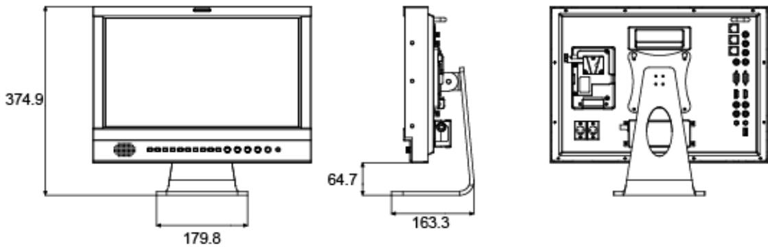
With 19-inch rack mount bracket (in mm)
